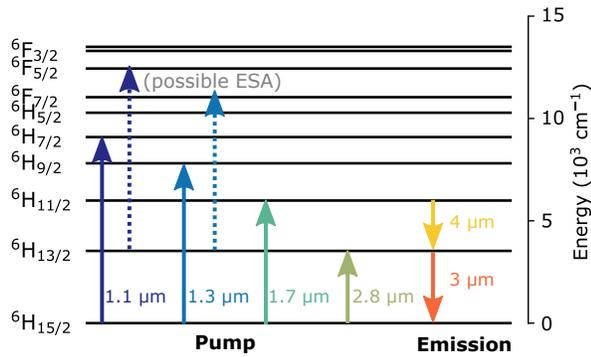
Fig. 2. Energy level diagram for dysprosium, showing possible pump and emission transitions with their corresponding approximate wavelengths (dotted lines indicate possible excited state absorption (ESA) transitions).
