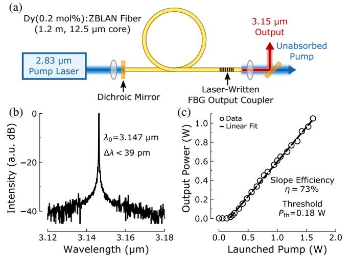
Fig. 3. Watt-level Dy:ZBLAN fiber laser: (a) setup; (b) optical spectrum; (c) power characteristic. Adapted from [14].
