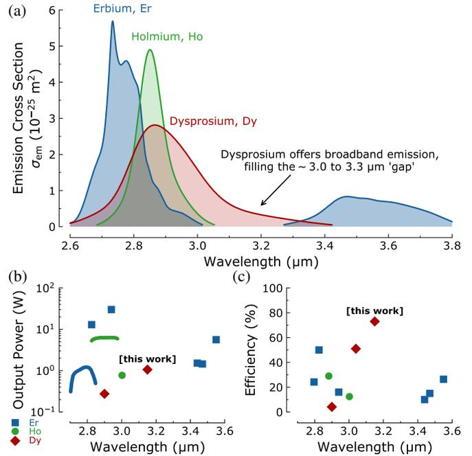
Fig. 1. State-of-the-art mid-IR fiber lasers: (a) emission cross-sections for Er-, Ho- and Dy-doped ZBLAN; (b) maximum reported output powers and slope efficiencies.
