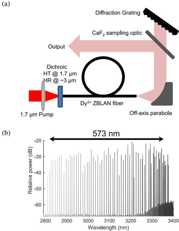
Fig. 4. Widely tunable Dy: fiber laser pumped at 1.7  $\mu\text{m}$ : (a) setup; (b) output spectra (tuned by rotating diffraction gratings). Adapted from [15].
