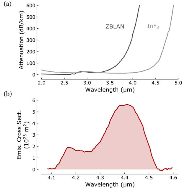
Fig. 5. (a) Comparison of attenuation in passive ZBLAN and  $\text{InF}_3$  fluoride fibers. (b) Measured emission cross section ( ${}^6H_{11/2} \rightarrow {}^6H_{13/2}$ ) beyond  $4 \mu\text{m}$  in Dy: $\text{InF}_3$  with  $1.7 \mu\text{m}$  pumping. Adapted from [25].
